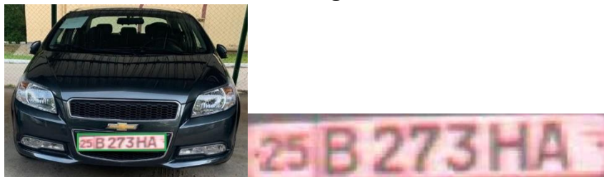
Figure 2. Car number identification: a) original image; b) allocated number plate
