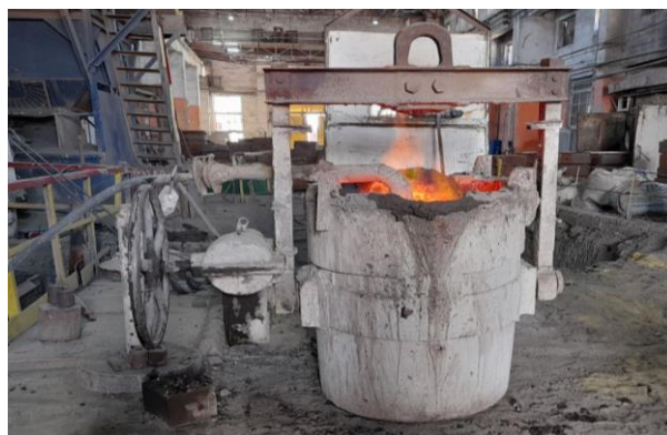
1 – picture. The process of heating the vessel using gas
