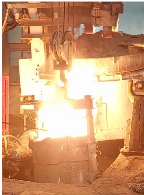
2 – picture. The process of loading liquid metal into a ladle
