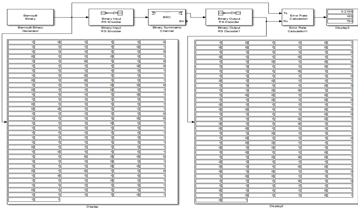
Fig.8. Scheme of the model of the error-correcting Reed-Solomon code in the digital television system of the DVB-T2 standard (error probability is 0.2)
