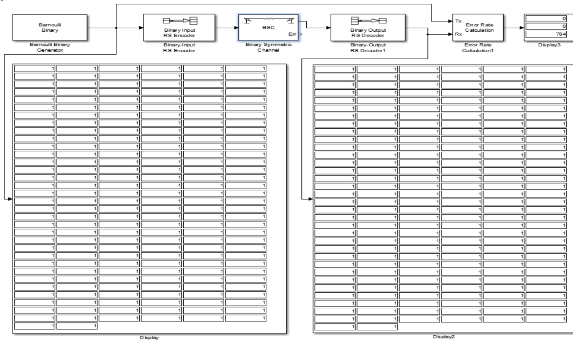
Fig.7. Scheme of the model of the error-correcting Reed-Solomon code in a digital television system of the DVB-T2 standard (error probability is 0)
