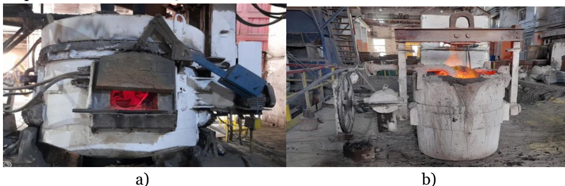
1 – picture. a) The process of loading ferroalloys into the furnace, b) The process of heating the furnace using a gas burner
